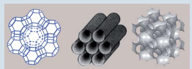
Schematic structure zeolite Y, MCM-41 and MCM-48 ( www.iza-structure.org , Nature 359 and 441)
